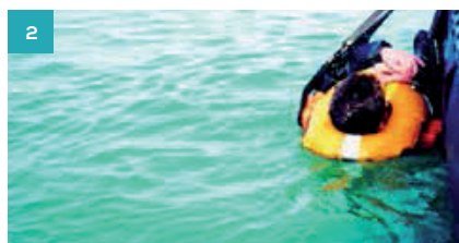
2 Due to the scoop configuration the casualty can be floated into the cradle with minimum effort.
